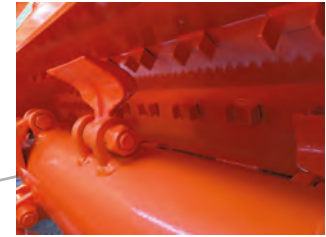
Hammers and internal debris catching lugs
