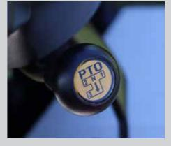
Convenience of a 3 speed PTO, 540 750 and 1000rpm. A speed for every job.
