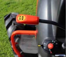
Well placed forward/reverse shuttle lever for ease
