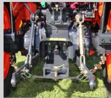
A rear lift capacity of 1131 kg. Standard with 2 sets A flat operator station, with a tilt steering column of rear hydraulic remotes.
