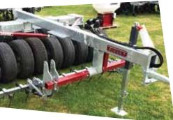
Front leading harrow option makes the tyre roller a more versatile machine.
