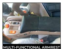
The multi-functional electronic armrest features numerous functions, such as throttle engagement, 3-point linkage lift and lower, Powershift and Auto Powershift mode.
