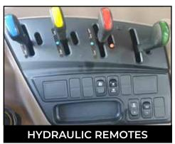
Changing or removing implements is light work on the HX, thanks to the four external rear hydraulic ports and one-handed quick couplers. Flow at the remotes is 118 L/min.
