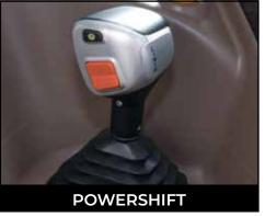
A simple button operation on the side speed lever and armrest gives you a 32x32 transmission with an 8-speed Powershift in 4 ranges.
