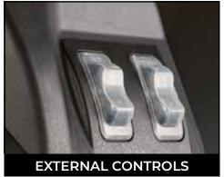
The addition of rear fender remote and PTO switches increases the convenience of both the removal and attachment of external implements.
