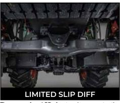
The use of a LSD front axle prevents the occurrence of slippage due to the load difference of the front wheels. This creates traction, greatly aiding manoeuvrability in any conditions.
