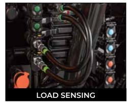
Load Sensing provides optimal hydraulic pressure and flow rate for load sensing operations. This results in automatically neutralising valves in the event of high loads during operation.
