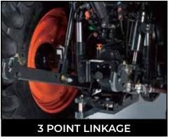
The electronic controlled 3-point linkage system boasts a 4852kg lifting capacity, allowing for the installation of multiple working implements.
