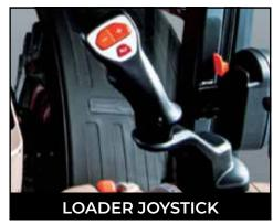
The multi-functional loader joystick is built with 3rd service and Powershift buttons, simplifying loader working conditions for the user.
